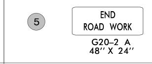
PLACE 500' FOLLOWING THE END OF CONSTRUCTION LIMITS OR AS SHOWN WHEN WORK ENDS AT A 3-WAY TEE INTERSECTION.
